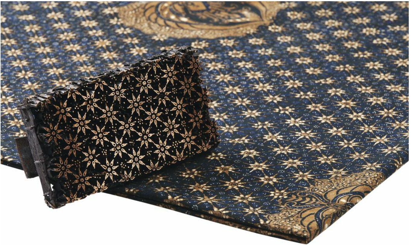
Figure 7 A metal stamp, canting cap , of the truntum design, resting on a cloth with the same stamped design. The wax would have been applied to both faces of the cloth (Private collection).
